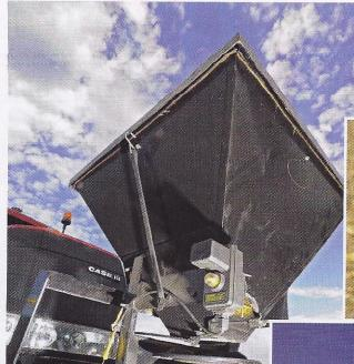
The spinner on the broadcast seeder is driven by an electric motor while an electric control valve is linked to a second slide gate added to the hopper. Push-button on/off control of this second gate is achieved through a switch in the tractor cab. Ryan Speer (front right) and Terry Jacob (front left) are quickly incorporating cover crops into their corn/soybean and wheat rotations, with help from Bill King (left rear) and Tom Spexarth.
